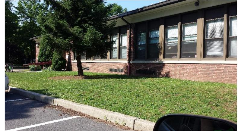
On the east side of the school, two rain gardens can be installed to capture, treat, and infiltrate roof runoff by disconnecting and redirecting adjacent downspouts. A preliminary soil assessment suggests that the soils have suitable drainage characteristics for green infrastructure.
